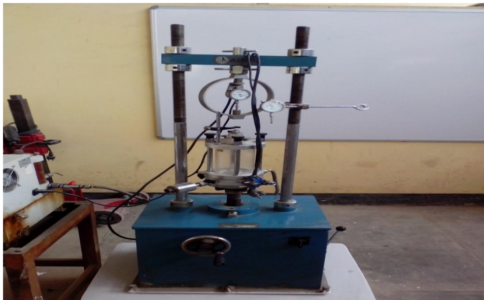
Fig. Tri axial apparatus set up.
