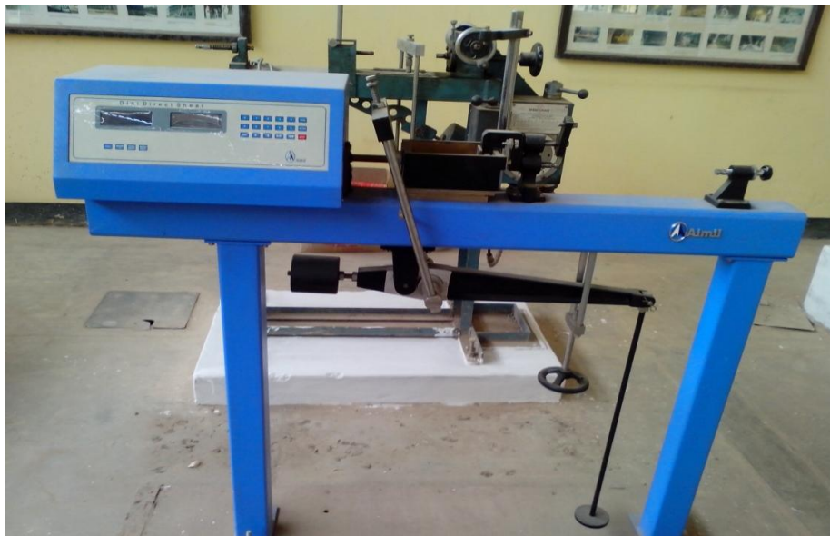
Fig. Direct shear apparatus set up.
