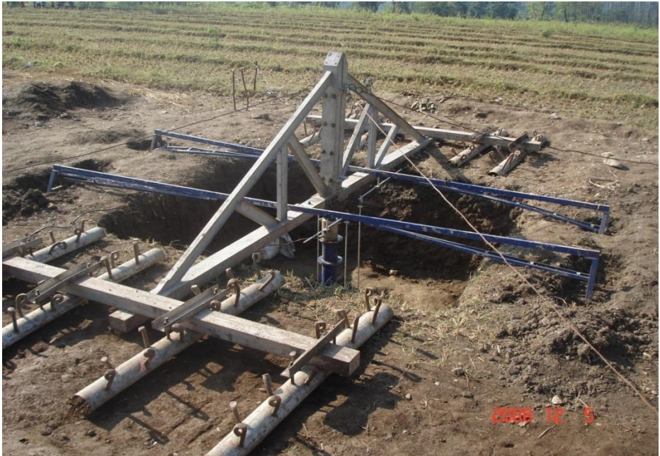
Fig. Plate Load test apparatus set up.
