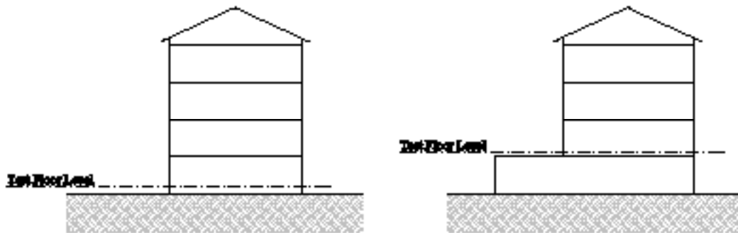
Figure. Test Floor Level in the case of regular building (on left) or building with singularities (on right)
